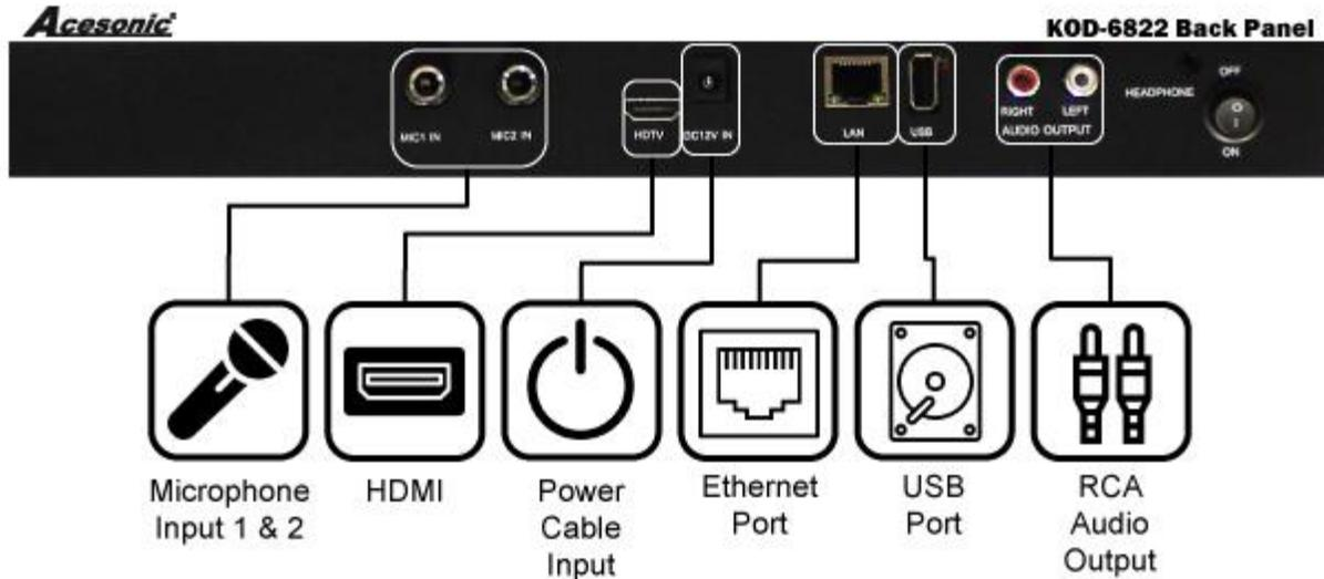
The KOD-6822 have multiple connectors on the back of the machine. In order to fully utilize the player, you must properly connect each port to the right device.
